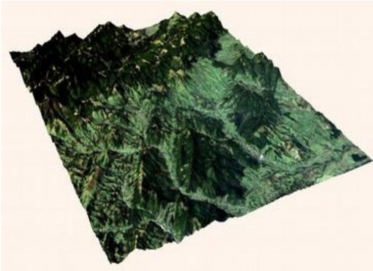
Figure 3 – An example of rendering a region of interest in 3D using Three.js: combination of elevation data from Terrain Tiles and a texture from Landsat 8, True Color, Carpathian Region, Ukraine
