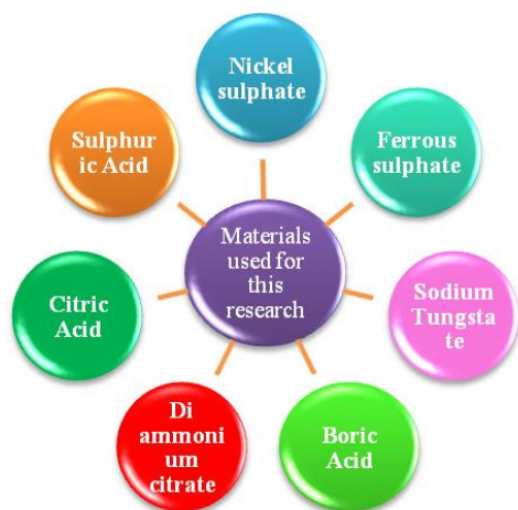
Fig. 6. Chemicals used for the electrodeposition of Ni-Fe-W alloy
