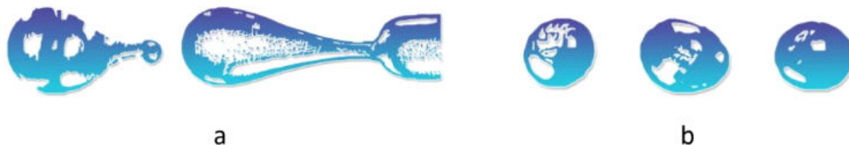
Fig. 3. Formation of uniform droplets without «companions» during the application of regular pressure pulses from an oscillating membrane to the jet (specific power 360 W/m 2 , f=584 Hz, d_{\text{canal}}=1.2 mm, pressure 0.54 m in water column meters, \lambda=6 mm): a – the first stage, formation of pear-shaped drops; b – the second stage, formation of spherical drops without «companions»
