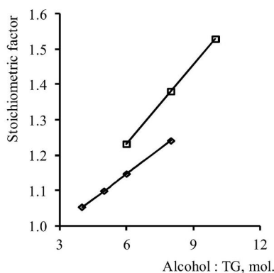
Fig. 7. The stoichiometric factor vs. the alcohol: triglyceride molar ratio: ◇ – ethyl alcohol, and □ – butyl alcohol
