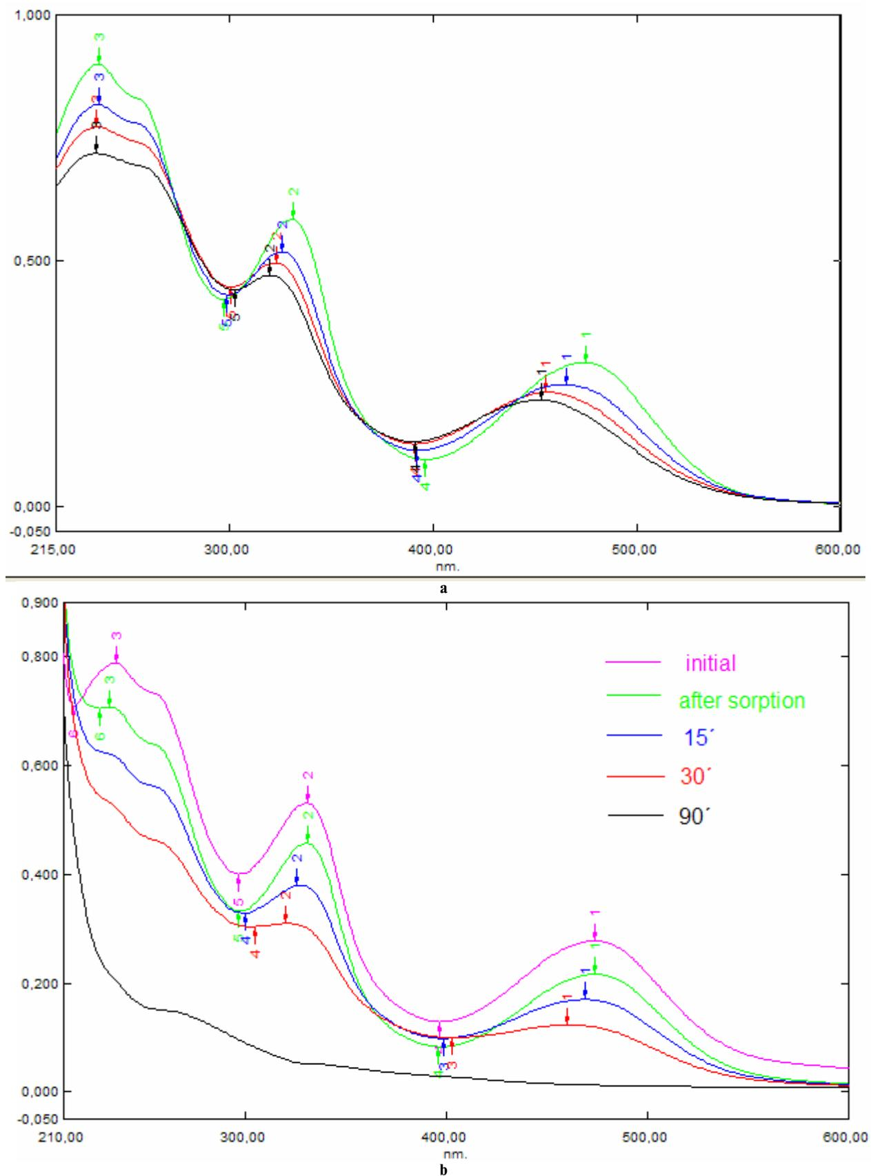
Fig. 4. Changes in the absorption spectra of RF water solutions under UV irradiation during 90 min: (a) photolysis, (b) over 0.5R
