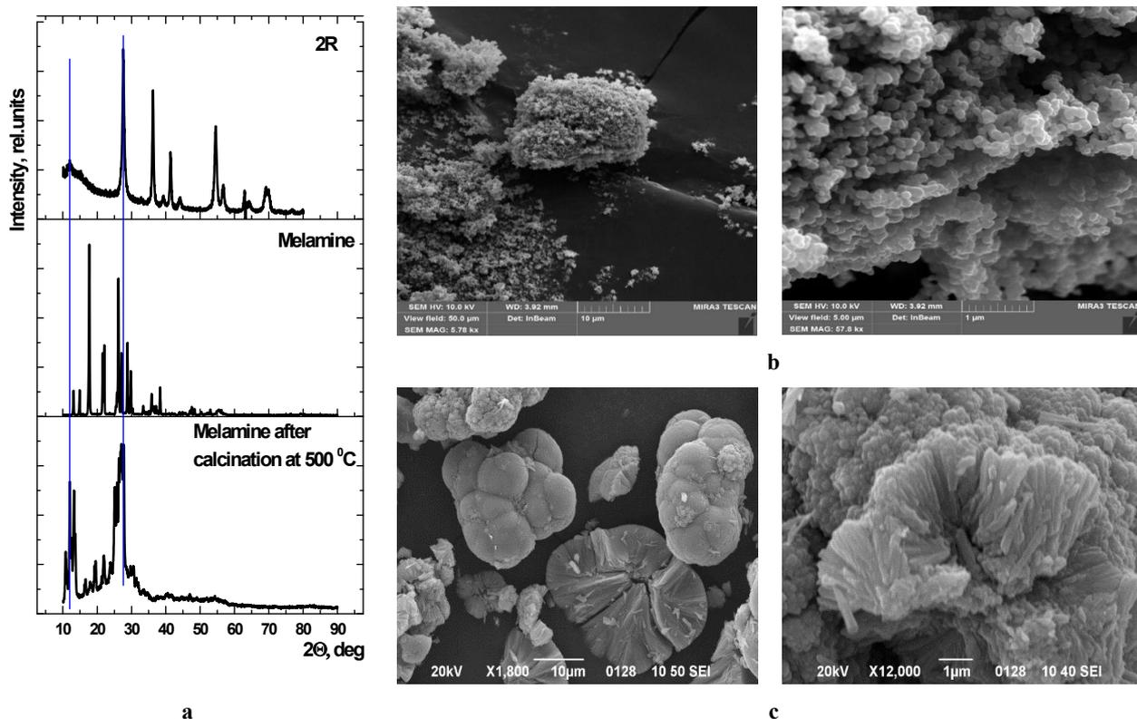
Fig. 1. XRD patterns of melamine, melamine after calcination at 500°C and 2R (a) and SEM image of 2A (b) and 2R (c)
