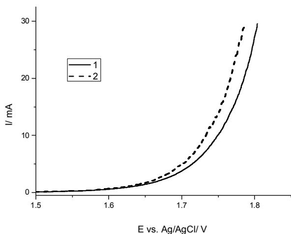
Fig. 3. Quasi steady-state polarisation curve for reduced Ti/TiO<sub>2</sub>-Pt nanotubes (1); thermal treated reduced Ti/TiO<sub>2</sub>-Pt nanotubes (2)
