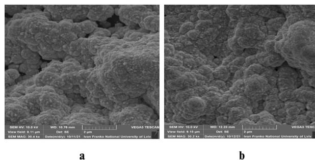
Fig. 2. SEM-images of following surfaces: a – reduced Ti/TiO<sub>2</sub>-Pt nanotubes; and b – thermal treated reduced Ti/TiO<sub>2</sub>-Pt nanotubes
