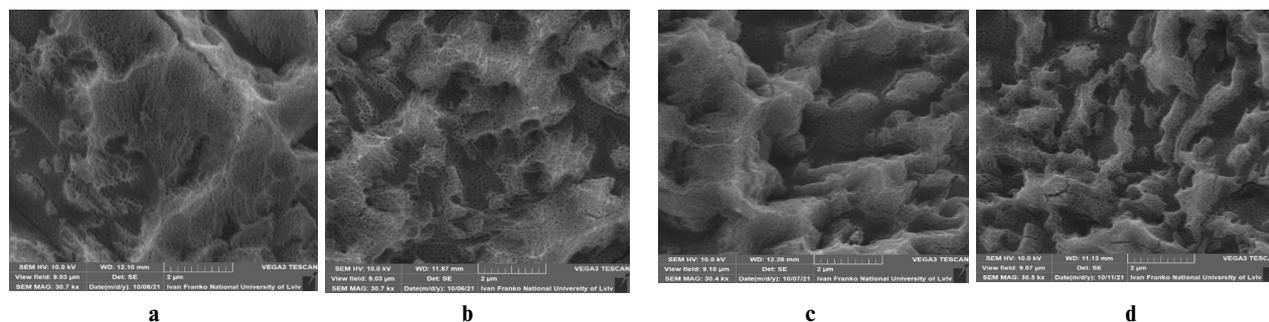
Fig. 1. SEM-images of following surfaces: a – Ti/TiO<sub>2</sub> nanotubes; b – thermal treated Ti/TiO<sub>2</sub> nanotubes; c – reduced Ti/TiO<sub>2</sub> nanotubes; and d – thermal treated reduced Ti/TiO<sub>2</sub> nanotubes
