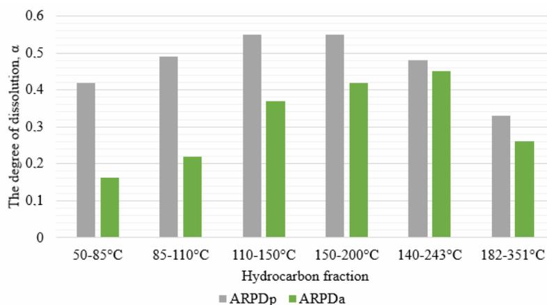
Fig. 1. The efficiency of light hydrocarbon fractions in dissolving ARPD in static mode
