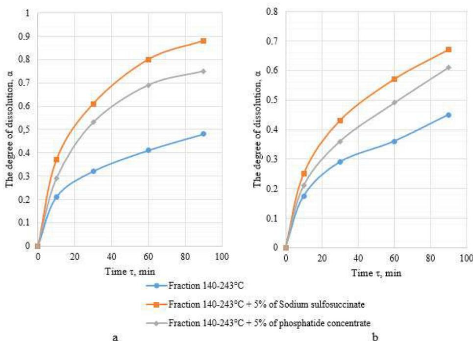
Fig. 3. The degree of dissolution of ARPDp (a) and ARPDa (b) in pure crude distilled fraction 140–243°C and in crude distilled fraction 140–243°C with 5 wt.% additives
