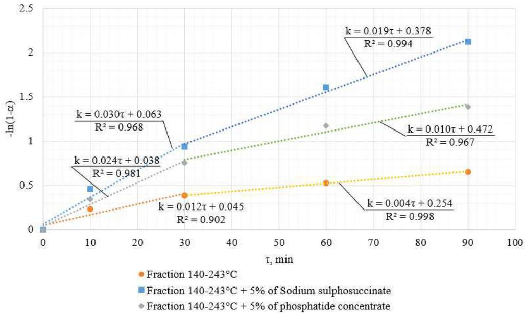
Fig. 5. Graphical determination of the constant of the dissolution rate of ARPDp in different solvents for the first and second stages of the process
