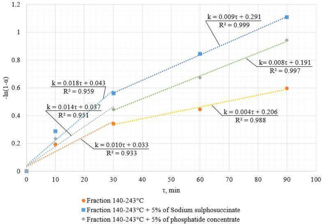
Fig. 4. Graphical determination of the constant of the dissolution rate of ARPDa in different solvents for the first and second stages of the process
