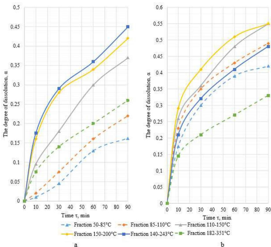
Fig. 2. Kinetic curves of dissolution of ARPDa (a) and ARPDp (b) in crude distilled oil fractions
