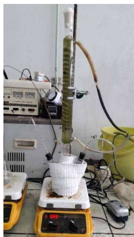
Fig. 2. The apparatus of OPEFB delignification
