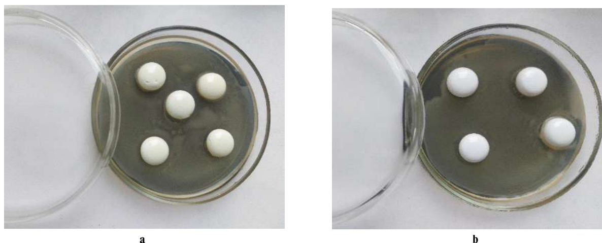
Fig. 1. Zone of growth inhibition of E. Coli biotest after contact with samples G-50Z (a) and G-50A (b)
